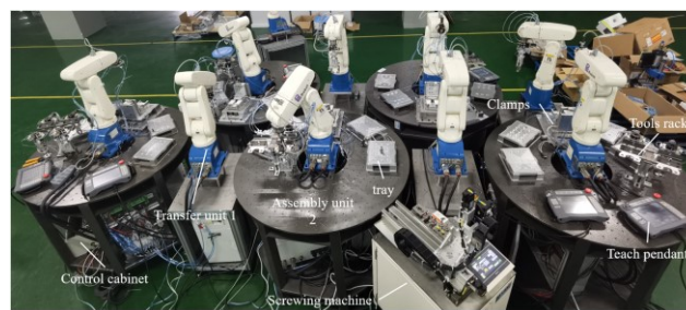
Fig. 1. An overview of the reconfigurable flexible assembly line.
